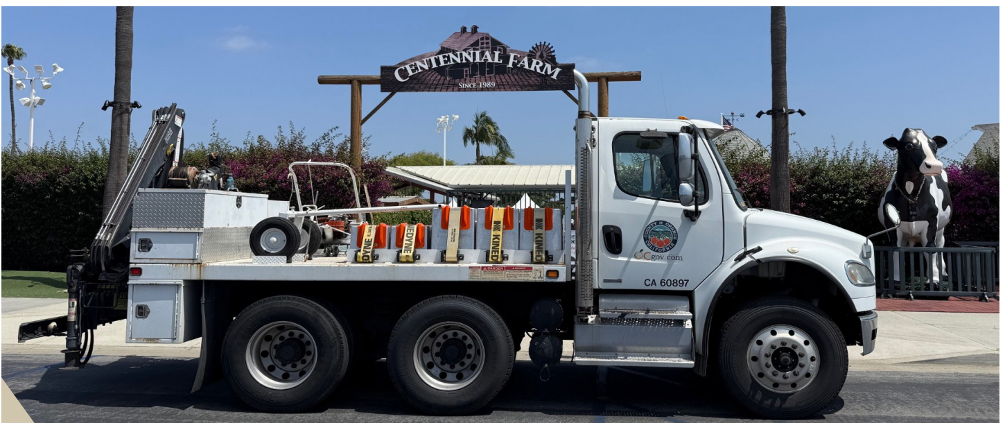
A livestock scale used for auctions at the County Fairgrounds is inspected using massive 500 and 1,000 pound standards.
