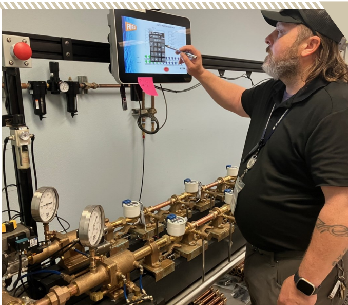
An electric submeter (above) and multiple water submeters (below) are being tested for accuracy at our on-site laboratory.
