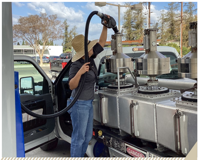
5-gallon provers are used to test all grades of gasoline at a retail fuel station.
