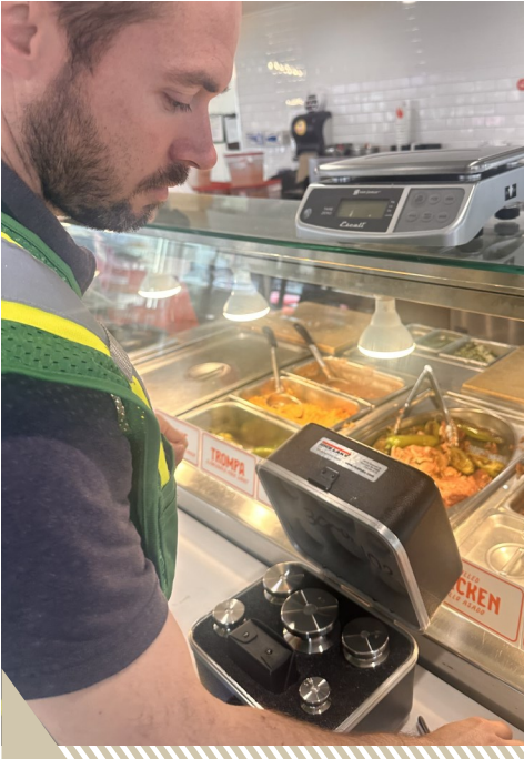
A grocery store deli scale is being tested using a 30-pound weight kit.
